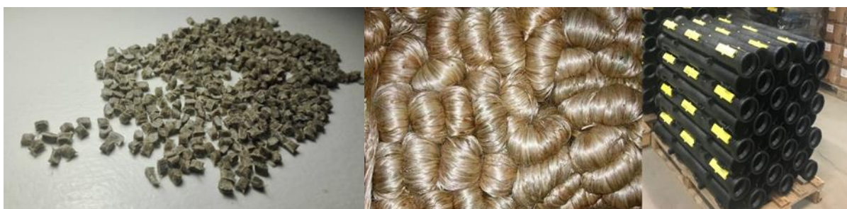
Figure 7. Jute granule and JuteSnap Split Pipe manufactured by JUTEBORG
